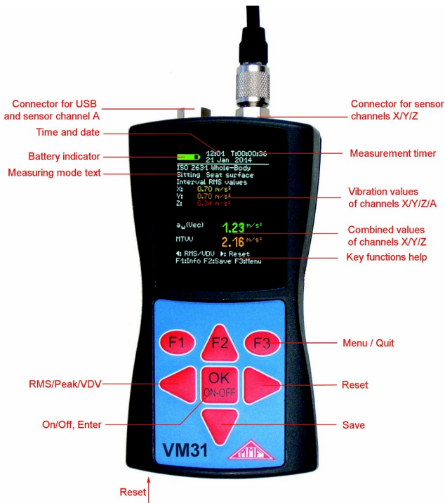
Figure 1: Controls, connectors and display
