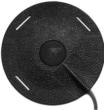
Figure 4: Seat pad accelerometer KS963B100-S
